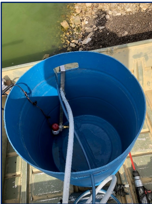
55-gallon drum and liquid air delivery system
